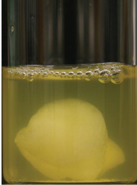
Figure 2.1: Typical coagulate complex (fibrin-hydrogel complex) formed after rotating a specific hydrogel composition (1.5 M APM, 1.5 M acrylamide, 0.3 M BIS) in human plasma (4 % (w/v) sodium citrate) for 18 hours. 300 mg of dried hydrogel were placed in 9 mL of plasma.
